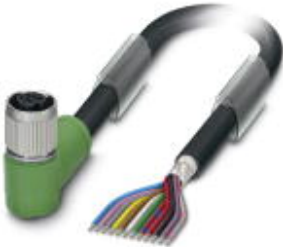
Sensor/Actuator cable, 12-position, PUR/PVC, Black RAL 9005, shielded, Free cable end, on Socket angled M12-SPEEDCON, A-coded, Cable length: 5 m
